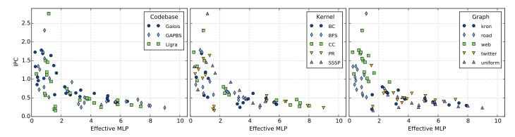
Fig. 4. Single-thread performance in terms of instructions per cycle (IPC) of full workload colored by: codebase (left), kernel (middle), and input graph (right).
