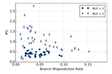
Fig. 5. Single-thread performance of full workload relative to branch misprediction rate colored by memory bandwidth utilization.
