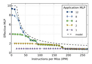
Fig. 2. Memory bandwidth achieved by parallel pointer chase microbenchmark with varying number of nops inserted (varies IPM). Using a single thread with differing numbers of parallel chases (application MLP).
