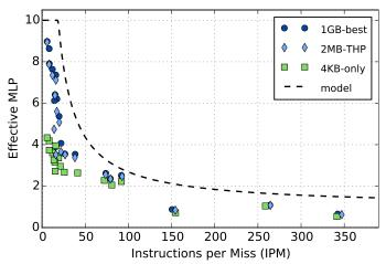
Fig. 8. Single-thread achieved memory bandwidth of GAPBS for all kernels and graphs varying the operating system page size. 2 MB-THP uses Transparent Hugepages (THP) and lets the operating system choose to promote 4 KB to 2 MB pages (happens frequently). 1 GB-best is the fastest execution using manually allocated 1 GB pages for the output array, the graph, or both.
