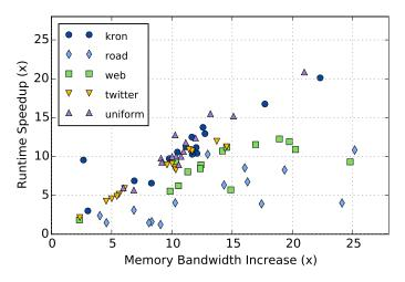
Fig. 9. Improvements in runtime and memory bandwidth utilization of full workload for full system (32 threads on 16 cores) relative to 1 thread. Points along unit slope transfer the same amount of data, so points below the unit slope (often road and web) transfer extra data.
